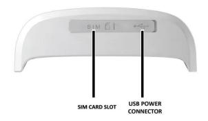
Open the rubber cover on the side of device ,insert the sim card into sim card slot , if you have purchased a MICRO SIM , you will need to use the Micro SIM adapter enclosed, like this:
